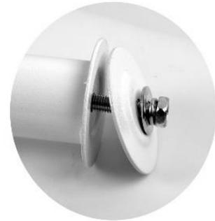
Cross the flat bars put the plate on the side with the wheels and insert the screw through.
